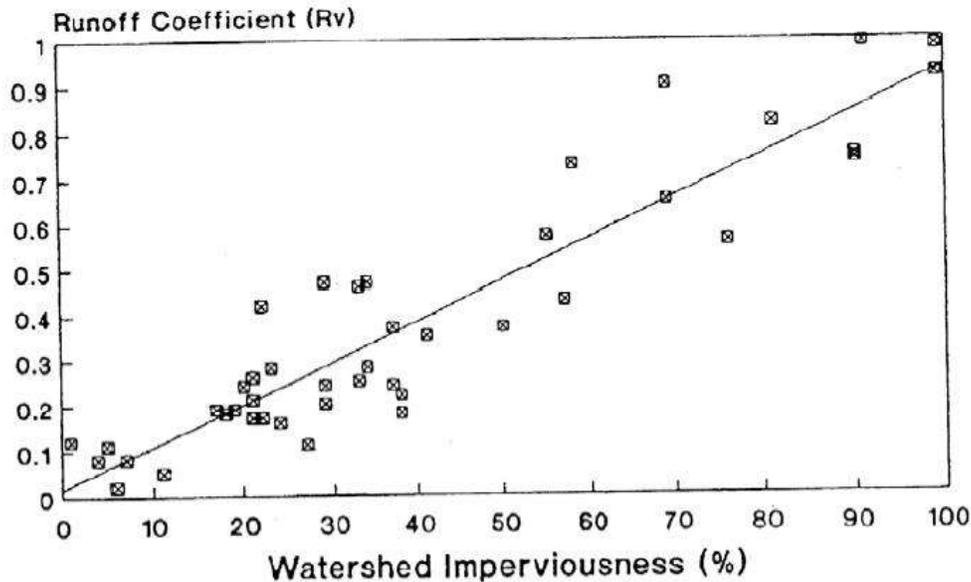
The increase in stormwater runoff can be too much for the existing local stormwater drainage system to handle. As a result, the stormwater drainage system is often “improved” to rapidly collect runoff and quickly convey it away (using curb and gutter, enclosed stormwater drainage pipes, and lined channels). The stormwater runoff is subsequently discharged to downstream receiving waters, such as the Alewife Brook and the Charles River in Cambridge.
